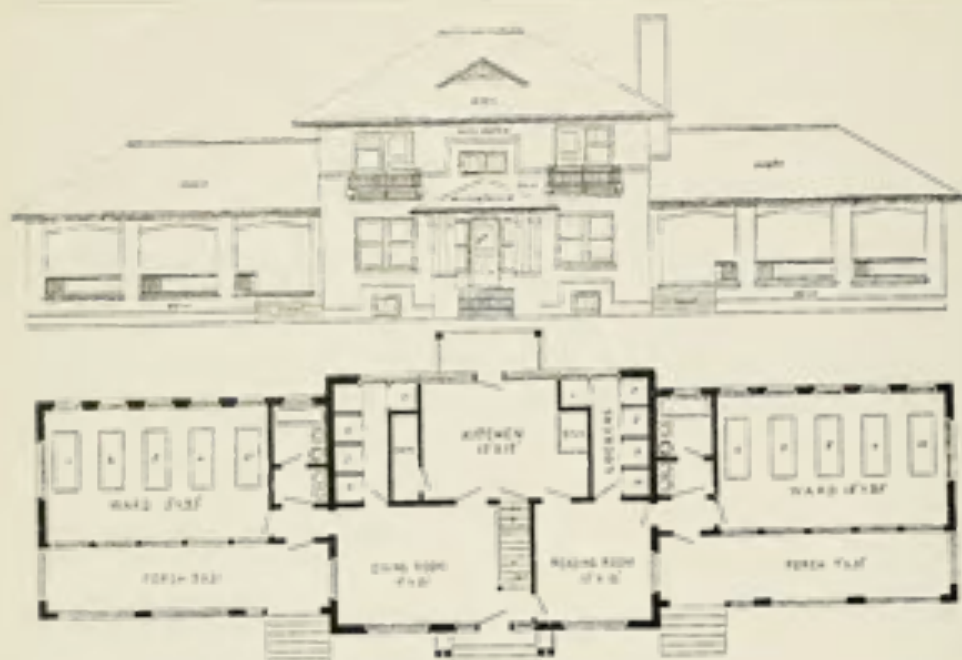
No. 44.—A Design for a Small Village or Town Hospital or Sanatorium. FRONT ELEVATION AND FLOOR PLAN. CAPACITY, 14 PATIENTS. ESTIMATED COST, $15,000.
