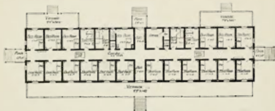
No. 53.—United States Army General Hospital, Fort Bayard, N. M. OFFICERS' QUARTERS. VIEW OF FRONT AND SIDE ELEVATION AND FLOOR PLAN. CAPACITY, 18 PATIENTS. COST, $18,534.
