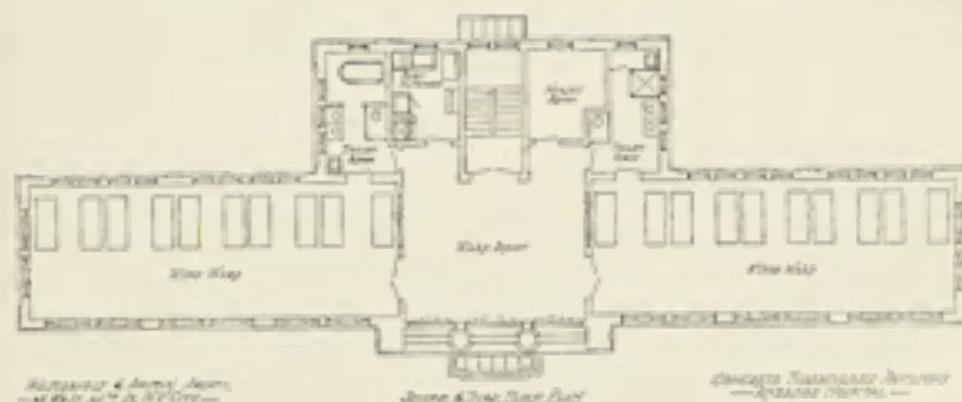
No. 48.—Riverside Hospital, New York City. DESIGNED BY DR. HERMANN M. BROGS. WESTERN & AUSTIN, ARCHT. CONCRETE PAVILION FOR ADVANCED CASES. FRONT ELEVATION AND FLOOR PLANS. CAPACITY, 75 PATIENTS. ESTIMATED COST, $40,000.
