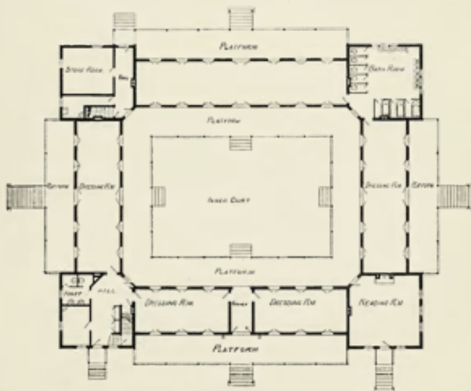
No. 54.—United States Army General Hospital, Fort Bayard, N. M. DESIGNED BY MAJOR GEORGE E. BUSHNELL. ENLISTED MEN'S WARD No. 2. VIEW OF FRONT AND SIDE ELEVATION AND FLOOR PLAN. CAPACITY, 32 PATIENTS. ESTIMATED COST, $25,000.
