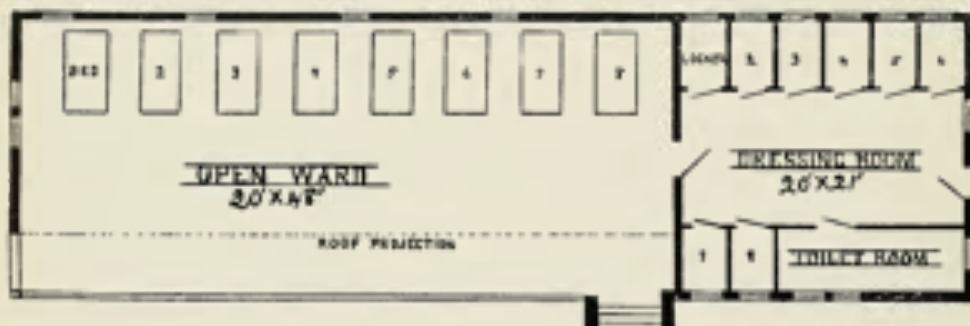
No. 91.—Loomis Sanatorium, Liberty, N. Y. DESIGNED BY DR. HERBERT MAXON KING, LEAN-TO. VIEW OF FRONT ELEVATION AND FLOOR PLAN. CAPACITY, 8 PATIENTS. ESTIMATED COST, $3,000. (See illustrations 1, 72, 73 and 108 for further description of this institution.)
