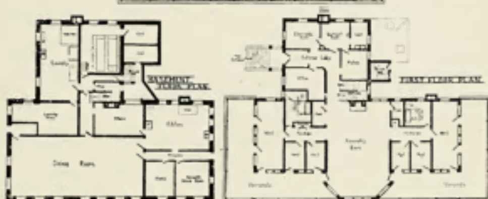
No. 25.—Manitoba Sanatorium, Ninette, Manitoba, Canada. DESIGNED BY DR. D. A. STEWART. ADMINISTRATION BUILDING. VIEW OF FRONT ELEVATION AND FLOOR PLANS. ADMINISTRATIVE CAPACITY, 100 PATIENTS. COST, $33,000. (See illustration 81 for further description of this institution.)
