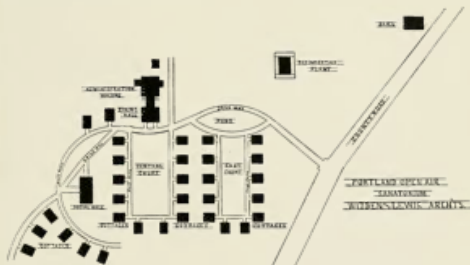
No. 8.—Portland Open Air Sanatorium, Portland, Ore. WHIDGEN & LEWIS, ARCHITECTS. BLOCK PLAN SHOWING METHOD OF GROUPING COTTAGES ABOUT OPEN COURTS AND THEIR RELATION TO THE ADMINISTRATION BUILDINGS AT A PRIVATE SANATORIUM. CAPACITY, 40 PATIENTS. ESTIMATED COST, $60,000. (See Illustrations 16 and 107 for further description of this institution.)
