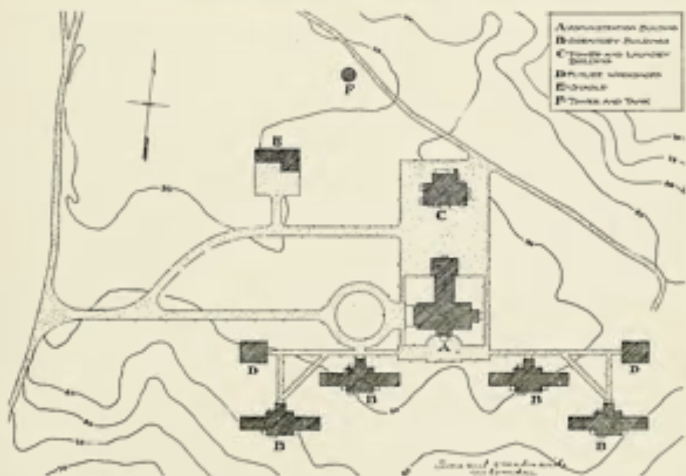
No. 12.—Preventorium for Children, Farmingdale, N. J. SCOPES & FEUSTMANN, AND WALTER W. JUDELL, ASSOCIATED ARCHITECTS. BIRD'S-EYE VIEW AND BLOCK PLAN SHOWING METHOD OF GROUPING THE BUILDINGS. (See illustrations 19, 27 and 93 for further description of this institution.)
