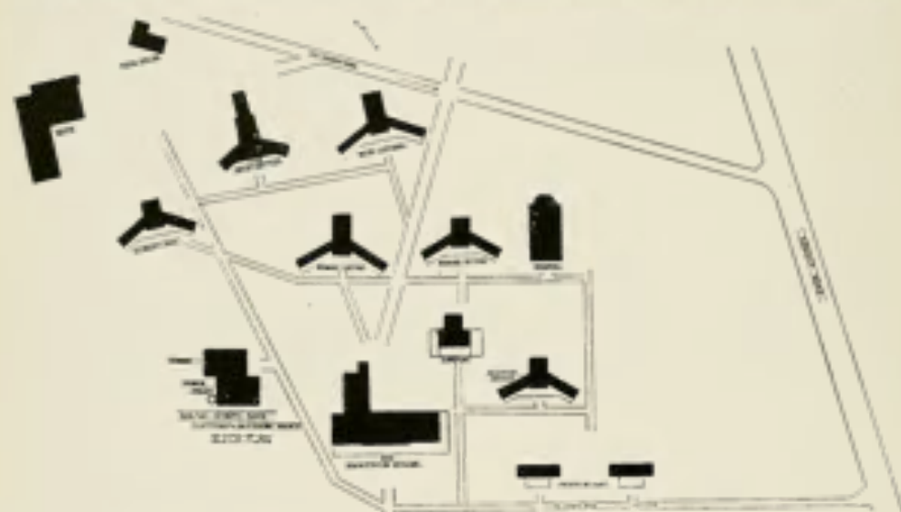
No. 11.—Maine State Sanatorium, Hebron, Me. T. C. STEVENS AND J. H. STEVENS, ARCHITECTS. VIEW AND BLOCK PLAN SHOWING METHOD OF GROUPING PAVILIONS IN THE REAR OF THE ADMINISTRATION BUILDING AND POWER HOUSE. CAPACITY, 100 PATIENTS. ESTIMATED COST, $130,000. (See illustrations 23 and 38 for further description of this institution.)
