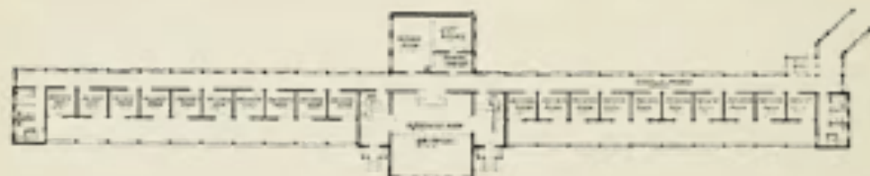
No. 51.—Indiana State Hospital, Rockville, Ind. WARD BUILDING. BRUNNER & STEEN, ARCHITECTS. VIEW OF FRONT ELEVATION AND FLOOR PLAN; BOTH FLOORS ALIKE. CAPACITY, 40 PATIENTS. ESTIMATED COST, $30,000. (See illustrations 7, 26 and 46 for further description of this institution.)
