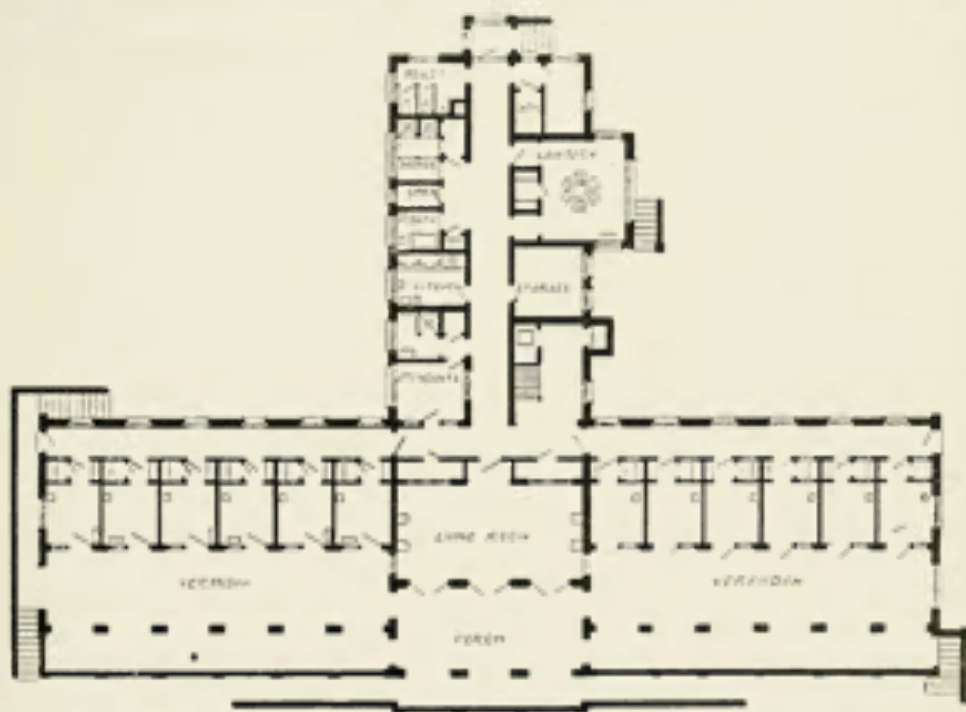
No. 67.—Ohio State Sanatorium, Mount Vernon, Ohio. F. L. PACKARD, ARCHITECT. RECEPTION HOSPITAL. VIEW OF FRONT ELEVATION AND FLOOR PLAN. CAPACITY, 24 PATIENTS. ESTIMATED COST, $30,000. (See Illustration 37 for further description of this institution.)
