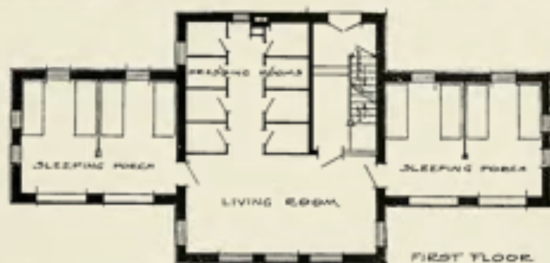
No. 14.—Municipal Sanatorium, Otisville, N. Y. DESIGNED BY DR. HERBERT M. BIGGS. JAMES D. BURT, ARCHITECT. SERVANTS' BUILDING No. 107. THIS STRUCTURE IS AN EXAMPLE OF A LEAN-TO CONSTRUCTED WITH FIRE-PROOF MATERIAL, DESIGNED TO SUPPLY OPEN-AIR SLEEPING QUARTERS FOR SERVANTS WHO WISH TO REHAB AND SUPPORT THEMSELVES AT THE INSTITUTION AFTER COMPLETING THE TREATMENT. CAPACITY, 16 PERSONS; COST, $5,000.
