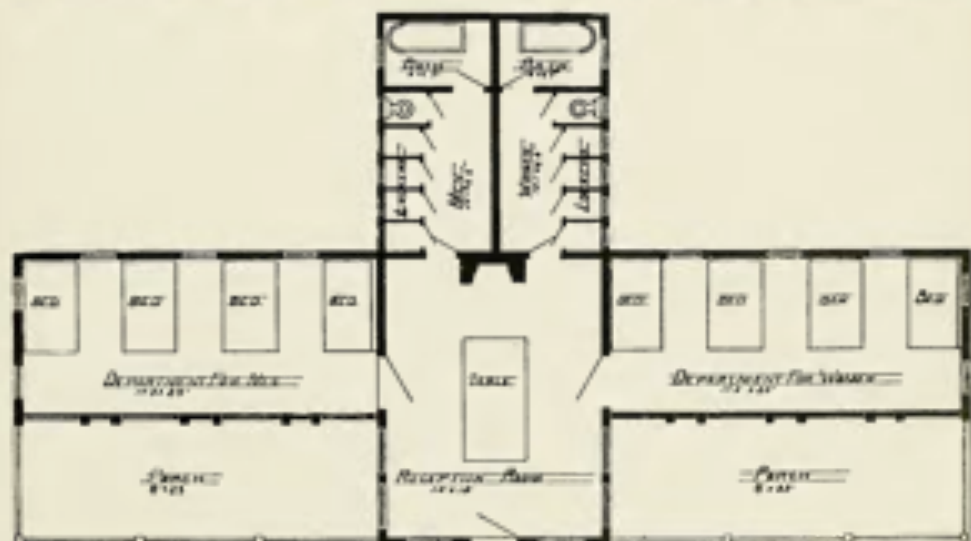
No. 76.—Delaware State Sanatorium, Wilmington, Del. J. & M. KENNEDY, ARCHITECTS. HERREW SOCIETY LEAN-TO. VIEW OF FRONT ELEVATION AND FLOOR PLAN. CAPACITY, 8 PATIENTS. ESTIMATED COST, $1,000.
