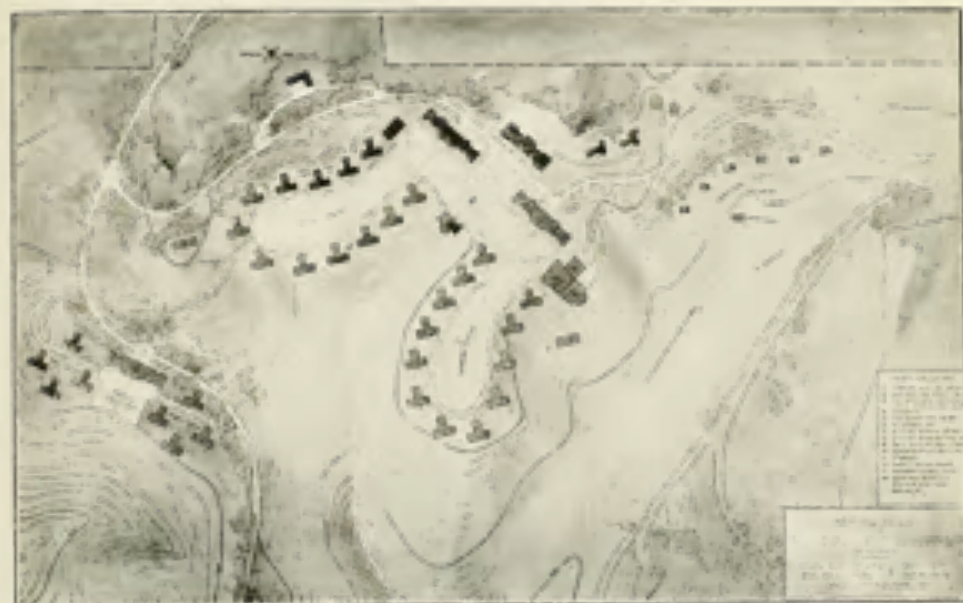
No. 4.—Georgia State Sanatorium, Alto, Ga. SCOTT & FEUSTMANN, AND WALTER W. JUDGILL, ASSOCIATED ARCHITECTS. BLOCK PLAN SHOWING THE CONTOUR LINES AND THE METHOD OF GROUPING THE LEAN-TO'S ON TWO PROMONTORIES IN FRONT OF THE ADMINISTRATION BUILDING. NOTE THE NEGRO QUARTERS ON THE LEFT OF THE ILLUSTRATION IN THE FOREGROUND. CAPACITY TO BE 400 PATIENTS. ESTIMATED COST, $175,000. (See illustrations 65 and 78 for further description of this institution.)
