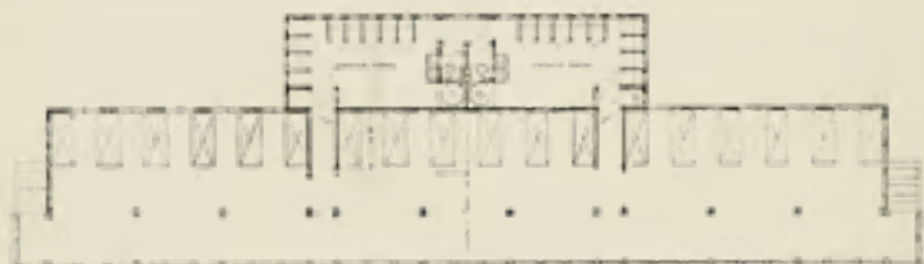
No. 85.—Municipal Sanatorium, Otisville, N. Y. DESIGNED BY DR. HERMANN M. BIGGS, JOSEPH B. VAN PELT, ARCHITECT. LEAN-TO. VIEW OF FRONT ELEVATION, AND FLOOR PLAN. CAPACITY, 18 PATIENTS. ESTIMATED COST, $4,400. (See illustrations 14, 28, 39, 60, 94 and 100 for further description of this institution.)
