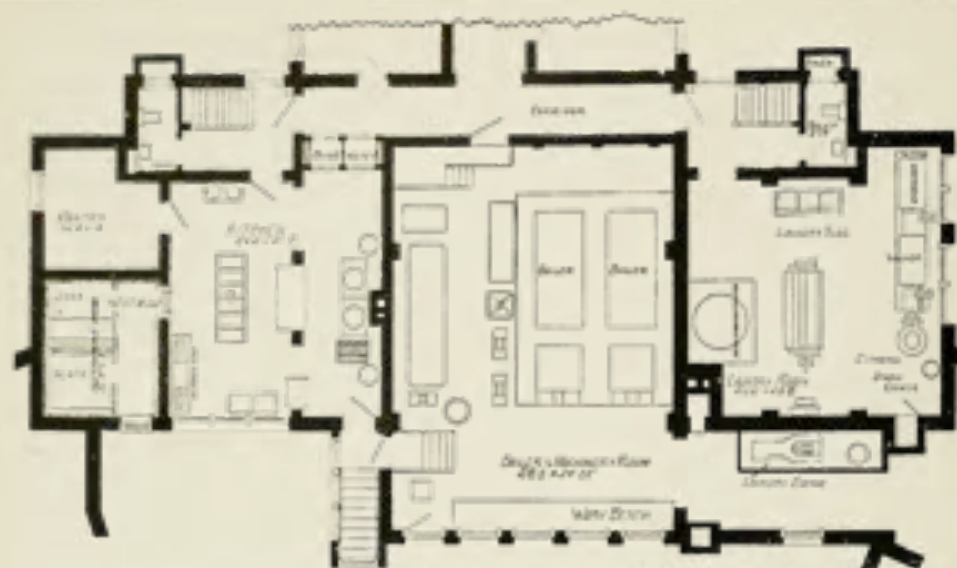
No. 20.—District Tuberculosis Hospital, Lima, Ohio. McLAUGHLIN & HULSKEN, ARCHITECTS. A PART OF THE BASEMENT FLOOR PLAN, SHOWING ARRANGEMENT OF LAUNDRY AND POWER PLANT, IN AN ADMINISTRATION BUILDING. (See illustration 43 for further description of this institution.)
