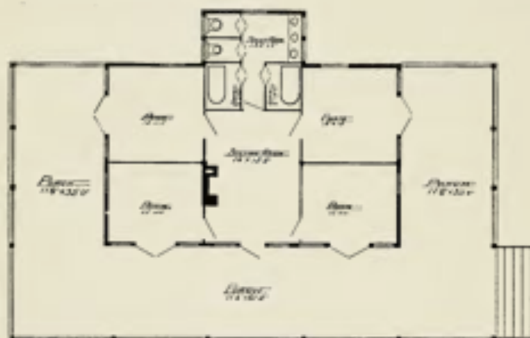
No. 99.—Association Sanatorium, Louisville, Ky. D. N. MURPHY & BROTHER, ARCHITECTS. COTTAGE. VIEW OF FRONT AND SIDE ELEVATION AND FLOOR PLAN. CAPACITY, 12 PATIENTS. ESTIMATED COST, $2,250.
