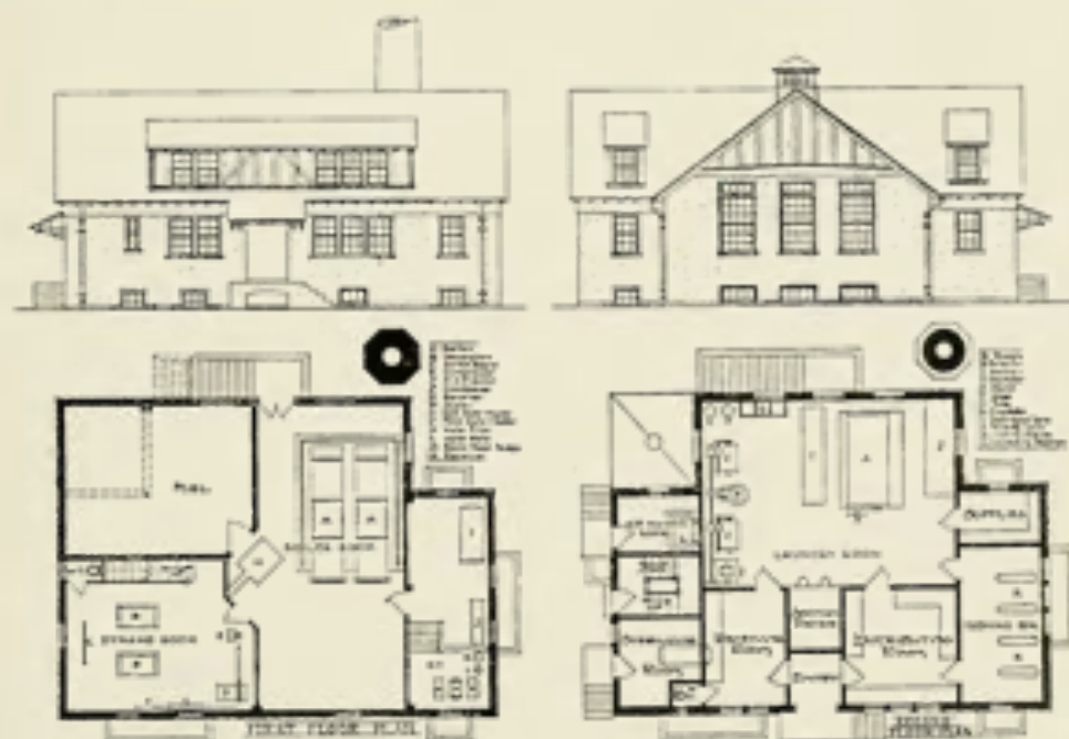
No. 19.—Preventorium for Children, Farmingdale, N. J. SCOPES & FEUSTMANN, AND WALTER W. JUDILL, ASSOCIATED ARCHITECTS. POWER HOUSE AND LAUNDRY. FRONT AND SIDE ELEVATIONS WITH FIRST AND SECOND FLOOR PLANS. (See illustrations 12, 27 and 95 for further description of this institution.)
