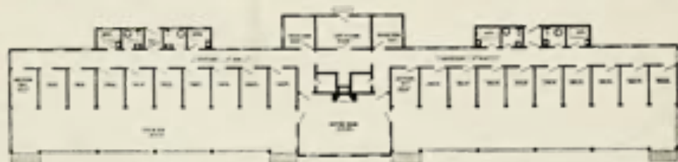
No. 64.—Maryland State Sanatorium, Sabillasville, Md. WYATT & NOLTING, ARCHITECTS. INFIRMARY BUILDING. VIEW OF FRONT ELEVATION, AND FLOOR PLAN. CAPACITY, 20 PATIENTS. ESTIMATED COST, $26,000. (See illustrations 3 and 73 for further description of this institution.)
